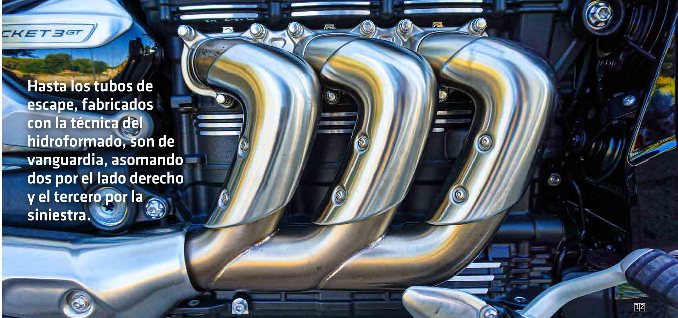
A close-up photograph of a motorcycle engine, specifically focusing on the exhaust system. Three large, polished stainless steel exhaust pipes are visible, arranged in a row. The pipes are hydroformed, giving them a smooth, curved appearance. They are mounted on the engine block, which is dark and metallic. The background shows various engine components, including a headlight and a fuel tank. The lighting is bright, highlighting the metallic surfaces and the intricate details of the engine.
